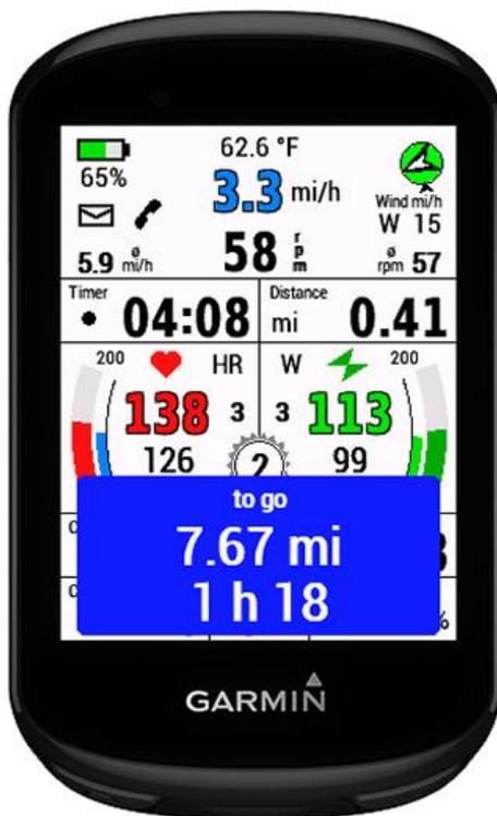
When a course is loaded, the data for time and distance to destination can be displayed at selectable intervals in a pop-up window.
