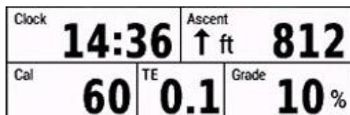
The bottom section of the display shows clock, Ascent, kcal Consumption, Training Effect and Grade or alternatively the Pause time (when paused).
